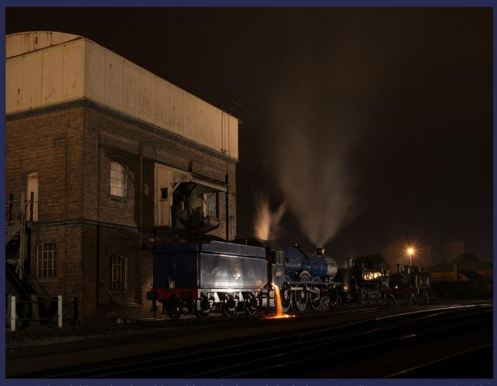
Aboce: It is the end of the working day and disposal duties take place on the last few locomotives still in steam. No. 6023 King Edward || has the clinker emptied from its firebox as preparations are made to add coal to the tender ready for the next turn. 8750 class 0-6-0PT Nos. 3738 and 1400 Class 0-4-2T No. 1466 await their turn on the ash pit. The evening was part of a Neil Cave photo charter on 29th June.
